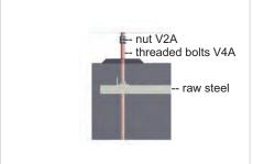
MATERIAL Anchor cage made of stainless
